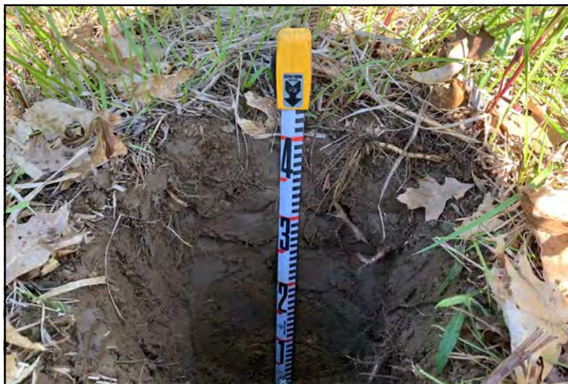
Photo 7. Example profile of an STP excavated in the remnant woodlot. Soils consist of an A-horizon of 32 cm of 10YR 3/2 silt loam over 10YR 5/6 sandy loam.
