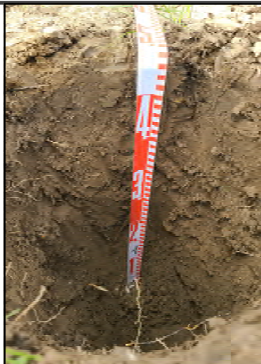
Photo 5. Example profile of an STP excavated in an area of previous construction disturbance. Soils consist of an A-horizon of 50 cm of 10YR 4/4 silt loam.
